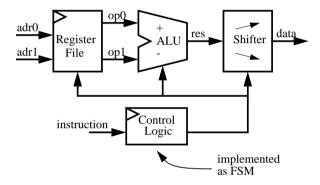
Finite State Machines (FSM) provide an easy-to-use model for defining, testing and implementing complex control circuits. They have been derived from the theory of finite automata. An FSM consists of a sequential part storing the current state of the machine in registers, and a combinational part for evaluation of the output signals and the next state from the input signals and the current state. The machine can change its state on every active clock edge.
