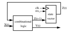
The next state and the outputs are both a function of the current state and the inputs:
