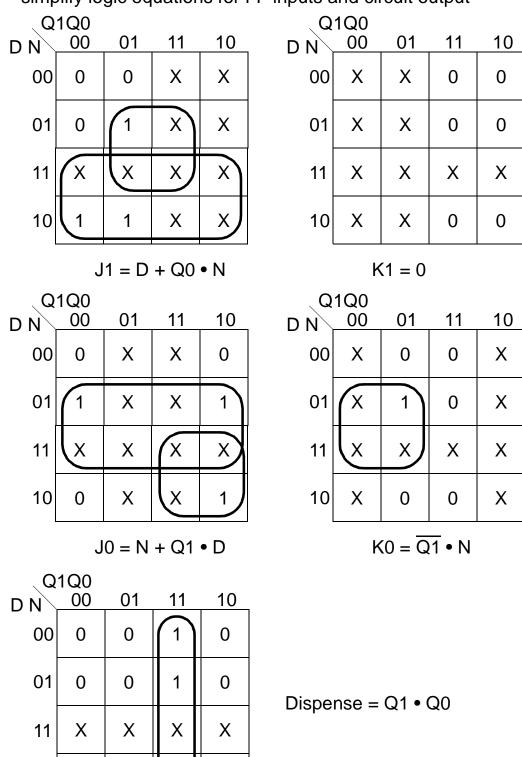
• simplify logic equations for FF inputs and circuit output
