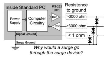
common mode surges. Plus surge diodes can add from 500 to 1000pf per wire -- remember RS-232 requires less than 2500pf per wire. Unless you can identify specific noise sources that would create normal mode spikes on your RS-232 wires, it may not be worth the signal distortion added by surge devices. If noise spikes are a real serious site problem, then you would be better off using a more robust standard like RS-422, modems with transformer isolation, or even fiber optics.
