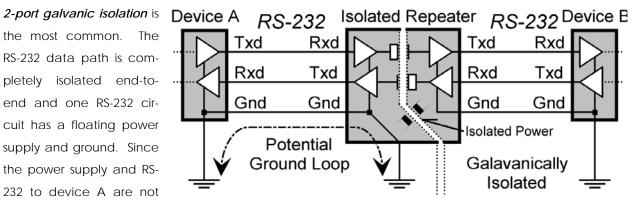
isolated, grounding problems can only be prevented by locating both in the same area and insuring both share a common ground path (one of the assumptions in the EIA/RS-232 standard). 2-port isolation does present another problem; if the isolated repeater shares a DC power supply with other devices, then surges in the common power supply will effect device A through the isolated repeater.
