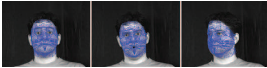
Figure 8: Three snapshots from the validation tracking sequence with contour-based refinement.
