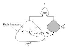
Figure 3: Circuit  $C_{\psi}^{ATPG}$  used for ATPG-SAT
