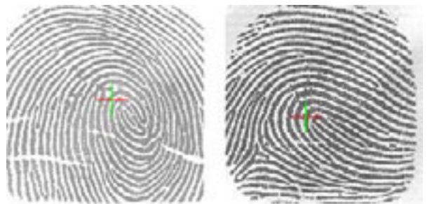
Figure 3. Results of core point detection based on single resolution method
