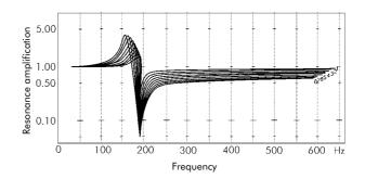
Figure 10 - Resonance curves of different detuned compensators ranging from 50 kvar (curve 1) to 400 kvar (curve 8), operated on a 1 250 kVA transformer (Frako)
