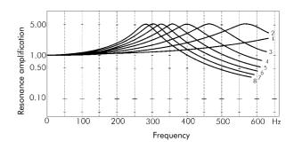
Figure 9 - Resonance curves of different compensators ranging from 50 kvar (curve 1) to 400 kvar (curve 8), operated on a 1 250 kVA transformer (Frako)
