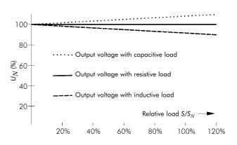
Figure 8 - Voltage drop in a transformer (here 630 kVA according to HD 428 list C) is minor under resistive load, major with inductive load and negative with capacitive load
