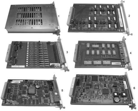
**Fig. 3** – Set of universal functional units (220×145 mm) arranged on separate printed boards, which different Nari-Relays MPDs consist of: PCS-931 (differential line protection), PSC-902 (distance protection), etc.
