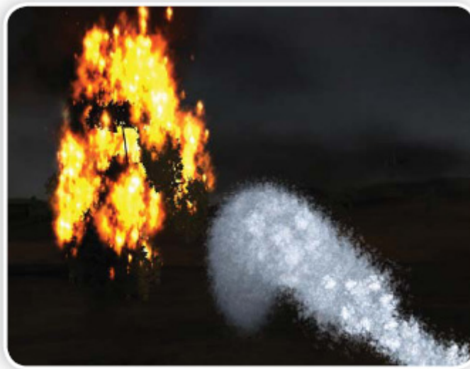
Fig.1. The fire system—water introduced as a cold emitter
