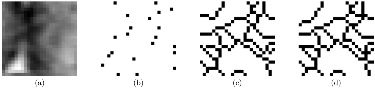
Figure 7. (a): original image, (b): minima of (a), (c): Meyer’s watershed line, (d): non-minima of the topological grayscale watershed
