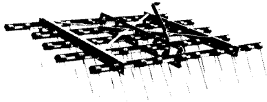
Figure 42 – Harrow—Section, round-wire teeth
