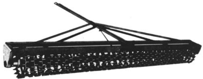
Figure 53 – Single packer roller—In-line roller gang—Drag-type pull hitch
