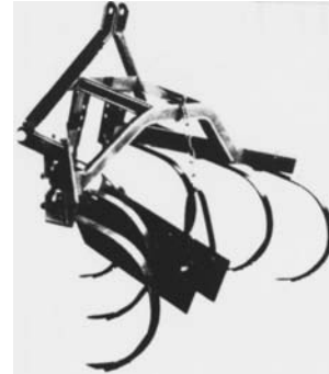
Figure 38 – Row crop cultivator—One-row, spring teeth, crop shields—Rear-mounted
