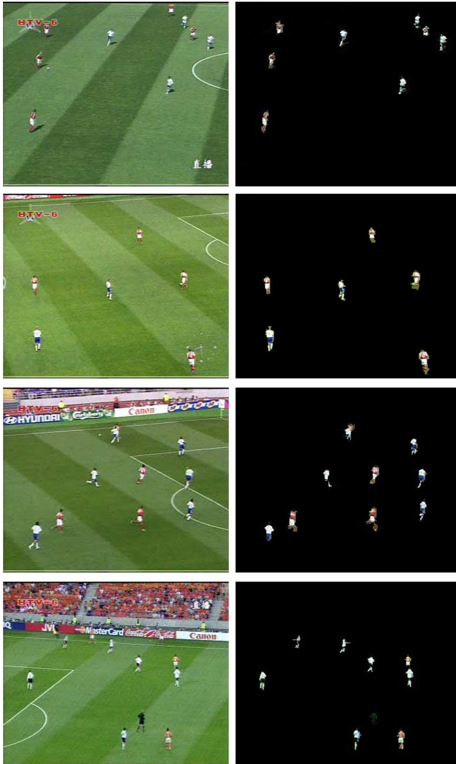
Fig. 6. The results of players segmenting are used to initialize the tracker for players. The left column are original images, and the right column are the segmented players.
