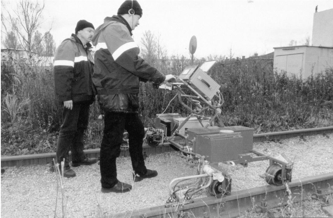
**Fig. 1.** AVIKON-01 flaw detector equipped with RI-01 data recorder.
