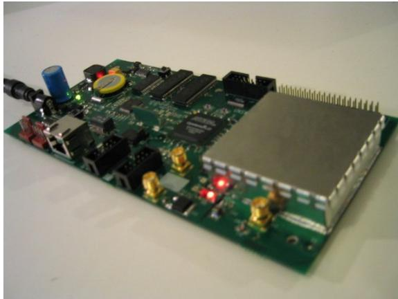
Figure 4 The new FPGA board
