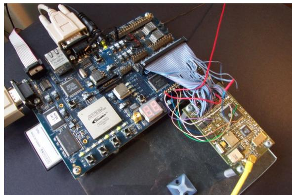
Figure 2 Modified Canadian Marconi SuperStar board interfaced to Altera Stratix development system.
