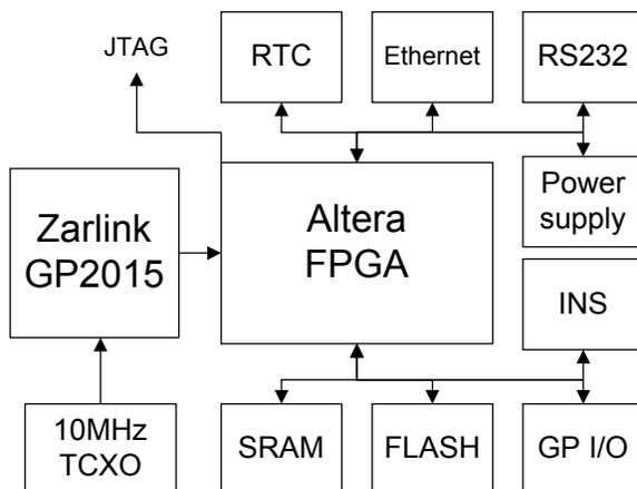
Figure 5 Main functions in the new FPGA receiver
