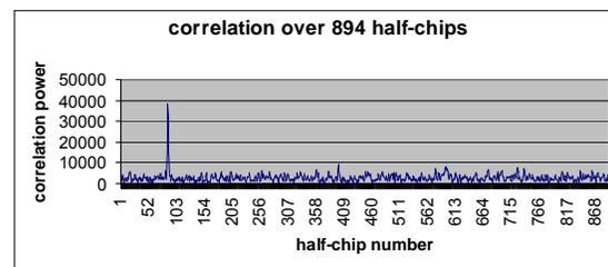
Figure 3 The first correlation from the FPGA receiver
