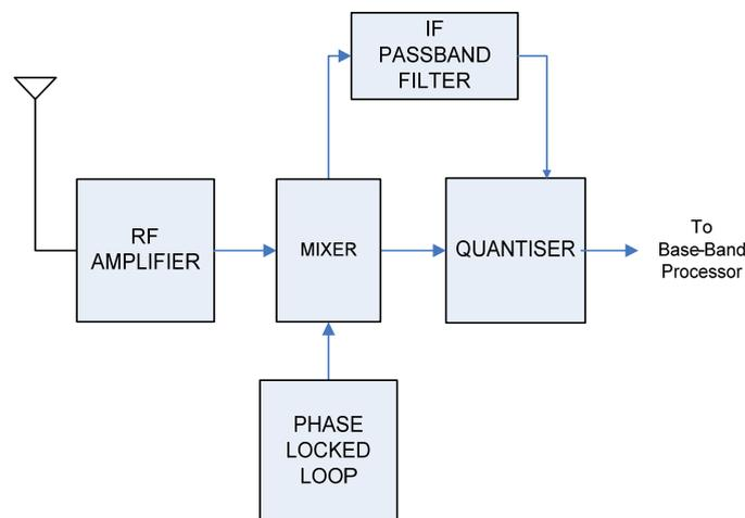
**Figure 1. GPS RF Front end architecture**
