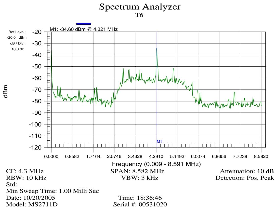
**Figure 3. Superstar II receiver with L1 signal at -96dBm**
