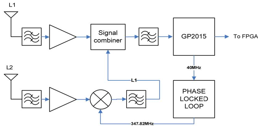
**Figure 5. L2 Front end converter**
