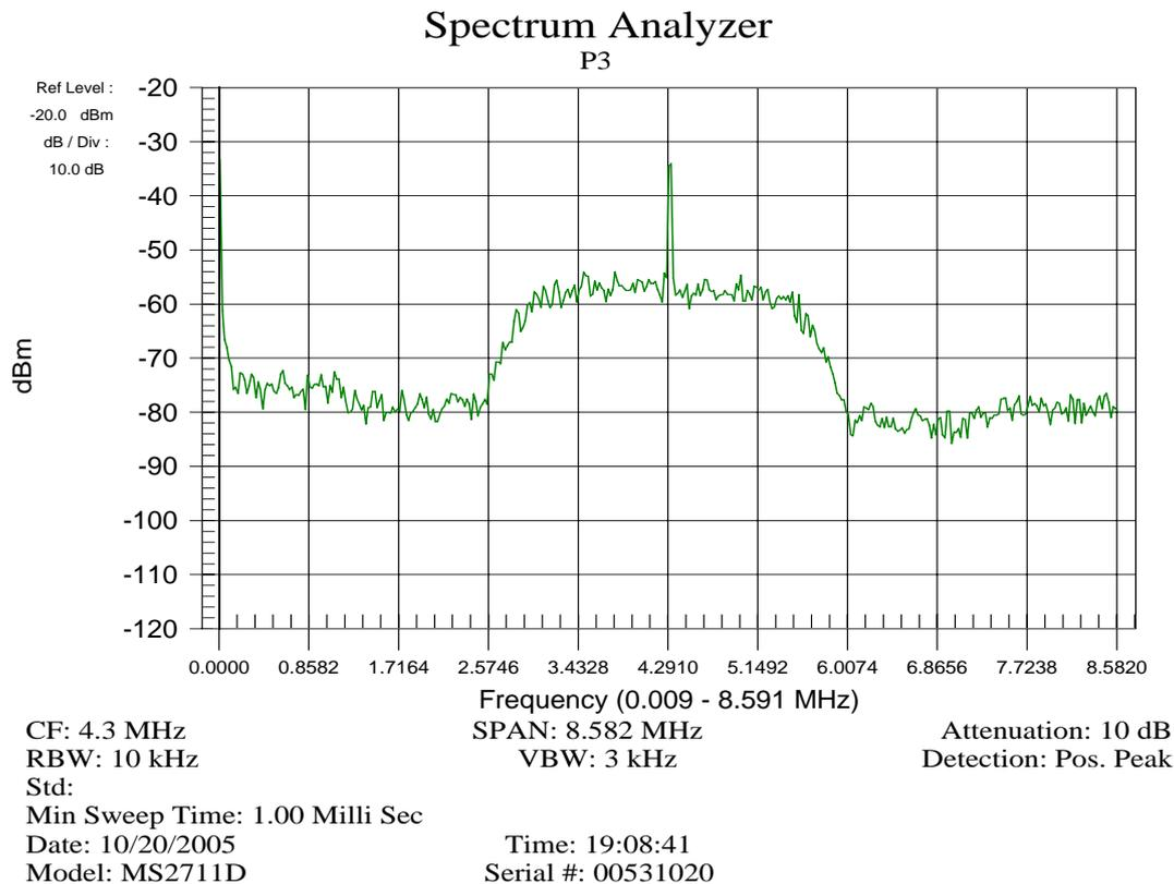
**Figure 3. Namuru receiver with L1 signal at -96dBm**
