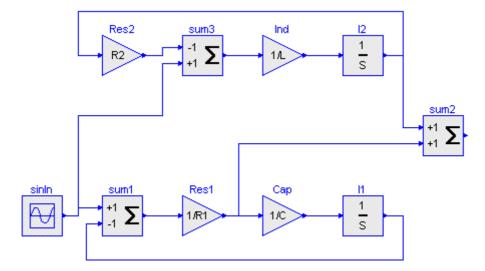
This example clearly shows the benefits of physically oriented, *non-causal modeling* compared to block oriented, causal modeling.
