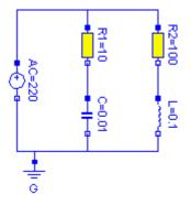
The system can be broken up into a set of connected electrical standard components. We have a voltage source, two resistors, an inductor, a capacitor and a ground point. Models of these components are typically available in model libraries and by using a graphical model editor we can define a model by drawing an object diagram very similar to the circuit diagram shown above by positioning icons that represent the models of the components and drawing connections.
