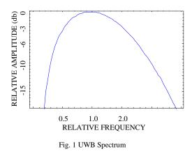
concept The series of impulses is transmitted at a repetition rate of up to several Megahertz. To convey information, the timing of individual pulses is altered to be either early or late corresponding to a digital "one" or "zero".
