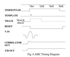
This ASIC device has been realized as a 3.0 mm by 3.8 mm flip-chip die using Silicon-Germanium (SiGe) technology. In this ASIC device the internal timing requirements and the 1 to 3 GHz operating frequency dictate the need for transistors having a minimum ft of 40 GHz. Additionally, the complexity of the device requires a low power technology to limit total power dissipation. SiGe offers all of these
