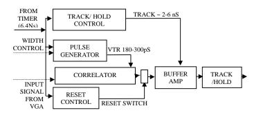
Fig. 5 Correlator Cell Block Diagram
