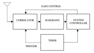
Fig. 3 UWB receiver block diagram
