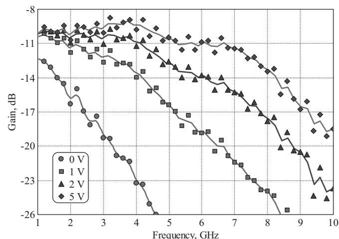
Fig. 3. Microwave gain of optoelectronic pair laser diode module – photodiode module versus frequency under different bias voltage of the photodiode.
