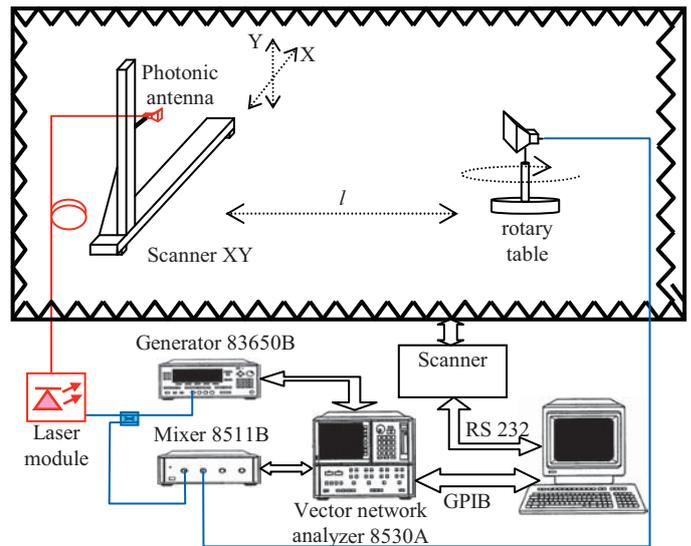
Fig. 7. Experimental set-up for the measurements of the photonic antenna gain
