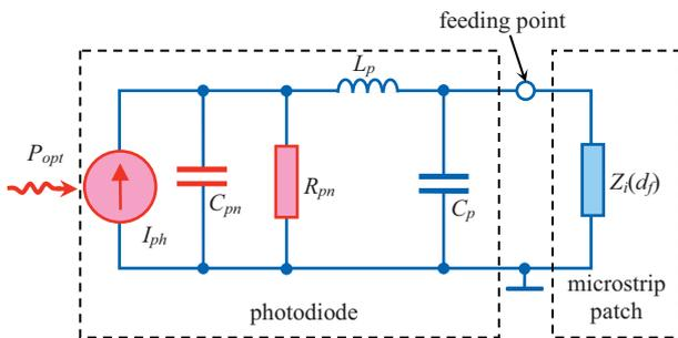
Fig. 6. Equivalent electrical circuit of the investigated active integrated photonic antenna for high frequencies
