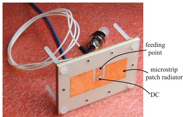
Fig. 4 Photo of the active integrated photonic antenna
