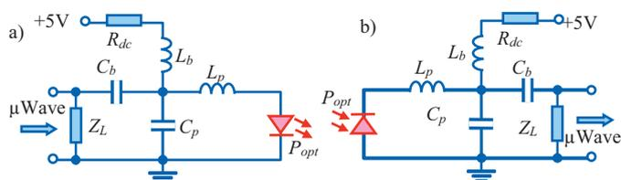
Fig. 2. Connection circuit of high-speed laser (a) and photodiode (b) modules.
