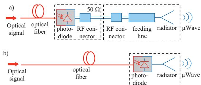
Fig. 1 Example of hybrid (a) and integrated (b) photonic antenna configurations
