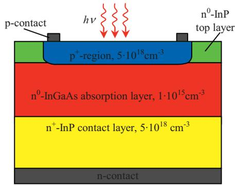
Fig. 5. Cross-section of the InGaAs/InP p-i-n photodiode
