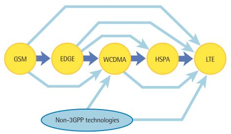
LTE provides a smooth evolutionary path for operators deploying all 3GPP and non-3GPP technologies.
