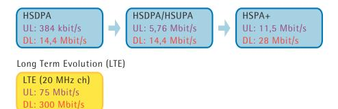
Uplink and downlink data rates compared for HSPA and LTE.
