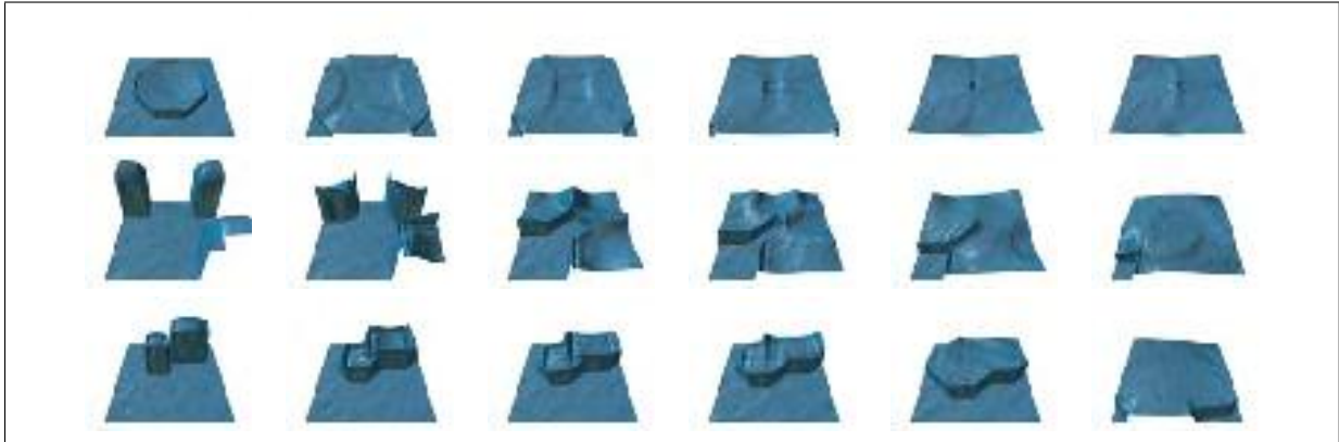
Plate 1: The pictures above are frames from rendering our shallow-water simulation, which uses our GPU-based tridiagonal matrix solver. Each row displays several frames from a different simulation, with the starting point of the simulation at the left. The top row simulates a 256 \times 256 grid, the middle row a 128 \times 128 grid, and the bottom row a 64 \times 64 grid. Thanks to Eric Lengyel for generating these images using his C4 game engine.
