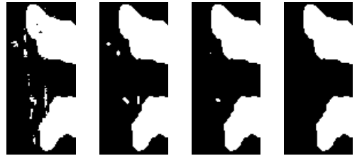
Figure 4: Segmentation result with different number of iterations j=0,2,4,6 (from left to right) during the MRF-computation.
