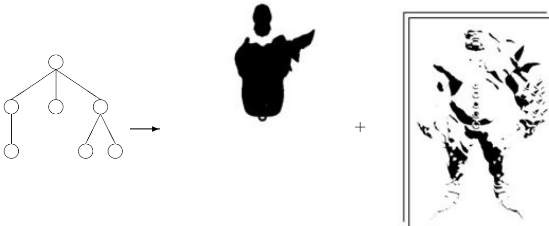
Figure 6: Render an octree and store the depth information in the depth buffer and the visual data (normals in this example) in a set of textures.
