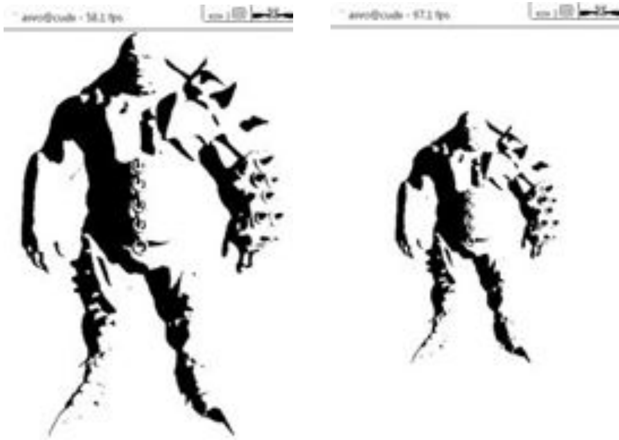
Figure 3: The frame rate increases as the projected size of the model decreases (58 fps vs. 97 fps), since the octree needs not be traversed as deeply to achieve the same visual quality.
