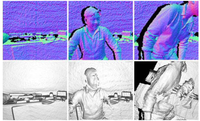
Figure 8: A user moves freely in front of a fixed Kinect. Live raw data (top) and shaded reconstruction (bottom). Left: Scene without user. Middle: User enters scene, but is only partially reconstructed due to motion. Right: Continued scene motions cause tracking failure.
