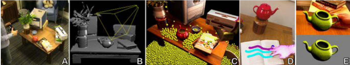
Figure 1: KinectFusion enables real-time detailed 3D reconstructions of indoor scenes using only the depth data from a standard Kinect camera. A) user points Kinect at coffee table scene. B) Phong shaded reconstructed 3D model (the wireframe frustum shows current tracked 3D pose of Kinect). C) 3D model texture mapped using Kinect RGB data with real-time particles simulated on the 3D model as reconstruction occurs. D) Multi-touch interactions performed on any reconstructed surface. E) Real-time segmentation and 3D tracking of a physical object.
