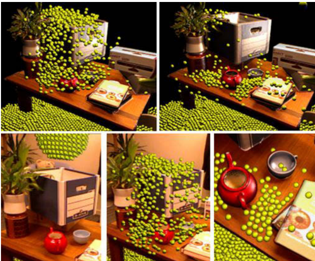
Figure 7: Interactive simulation of physics directly on 3D model even during reconstruction. Thousands of particles interact with reconstructed scene. Reconstruction, camera tracking, and physics simulation all performed in real-time.
