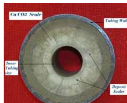
Figure 11 Sample of scale deposit in oil tubing from Libya
