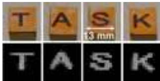
Fig. 10. Flipped photographs of rubber stamps and their tactile images captured by the fabricated tactile sensor module.
