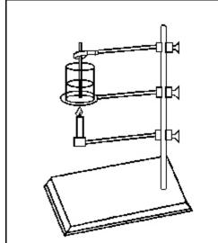
**Figure 2.** Set-up for determining the heat of combustion of a candle.
