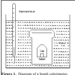
Figure 1. Diagram of a bomb calorimeter.
