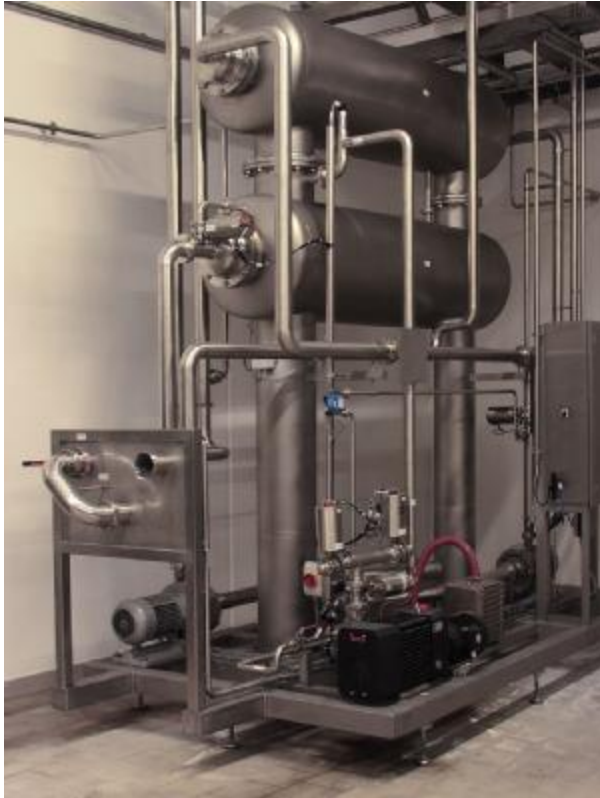
The DIOX two-stage vacuum deaeration plant consists of two horizontal vessels arranged one above the other, a vacuum pump, a circulating pump and an extractor pump. (Photos and table: GEA Diessel)
