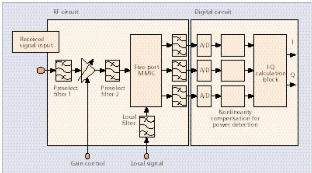
■ Figure 4. A block diagram of Sony CSL's SDR platform (SOPRANO).
