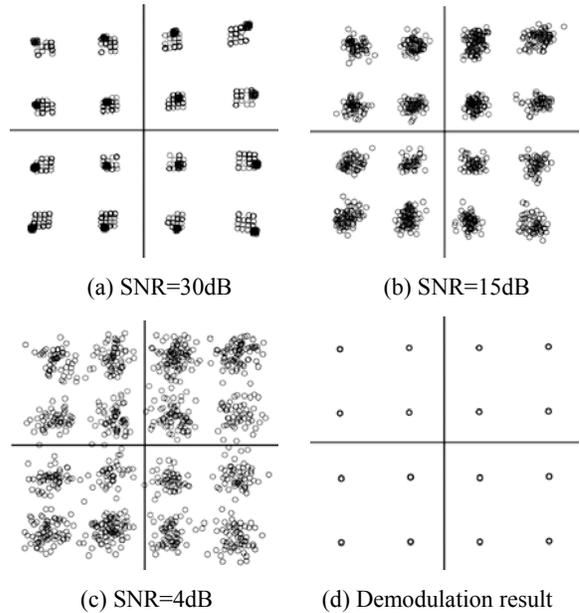
Fig. 6 Simulated output signal constellations for QAM16 with different SNR.
