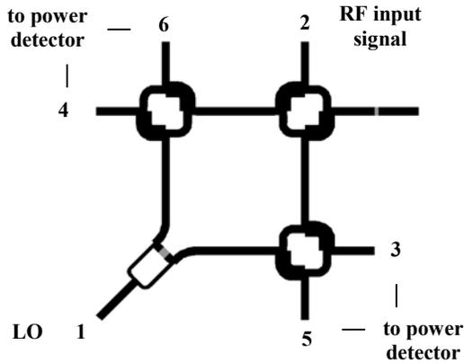
Fig. 3 Design layout of the six-port circuit
