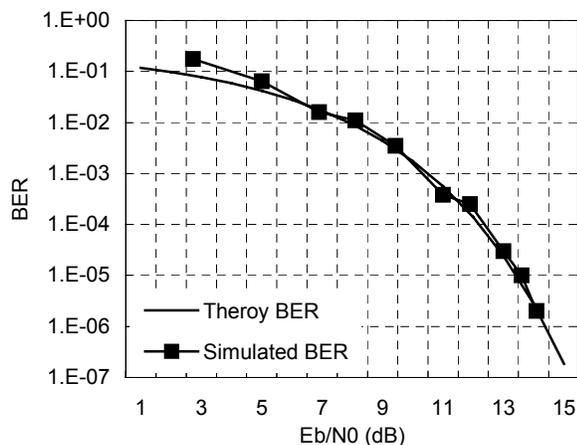
Fig. 8 Simulated and predicted BER for QAM16 modulation.
