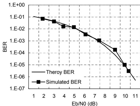
Fig. 7 Simulated and predicted BER for QPSK modulation.
