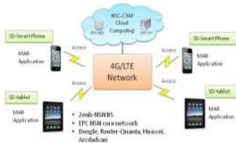
Figure 1. The experimental cloud-based 4G/LTE network testbed
