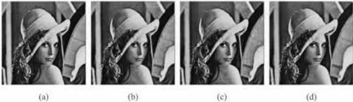
Fig. 8. Comparison of optimal wavelet functions for image Lena (PSNR = 36 dB). (a) Original. (b) DW-5 (PQS = 2.93). (c) CW-3 (PQS = 3.10). (d) BW-2.2 (PQS = 3.20).
