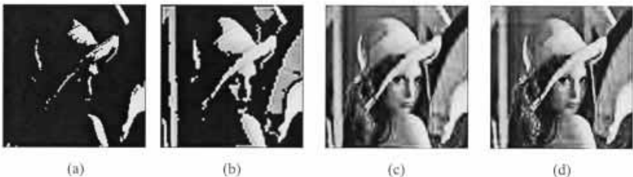
Fig. 6. Reconstructed image Lena; DW-5; CR = 50:1. (a) J = 1 (PSNR = 8.40 dB). (b) J = 2 (PSNR = 11.76 dB). (c) J = 3 (PSNR = 23.39 dB). (d) J = 4 (PSNR = 24.40 dB).
