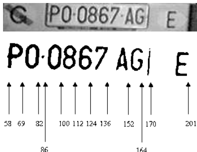
Figure 8. False character “E” is erased (the character comes from a country label, above image).
