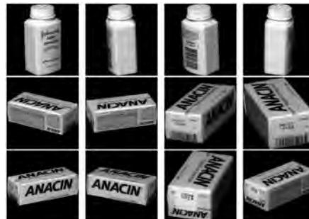
Fig. 10. Prototype views selected for two different 3D objects from the COIL data set using the algorithm described in Section 5.2. With this approach, views are allocated adaptively depending on the visual complexity of an object with respect to viewing angle.
