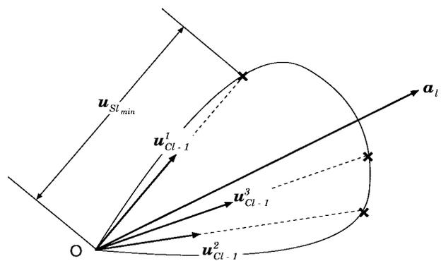
Fig. 11. SOFT adjusts the S-cell's selectivity to ensure the smallest output, in response to a training vector, is equal to  $u_{Sl_{min}}$ . Note the increased response of the S-cell to the second and third training patterns.
