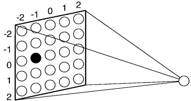
Fig. 3. The weight sharing mechanism used in the neocognitron makes it convenient to specify a particular connection in terms of  $\nu$ , the position of a source cell within a destination cell’s input region. In this  $5 \times 5$  cell input region the black cell is at  $\nu = (-1, 0)$ .
