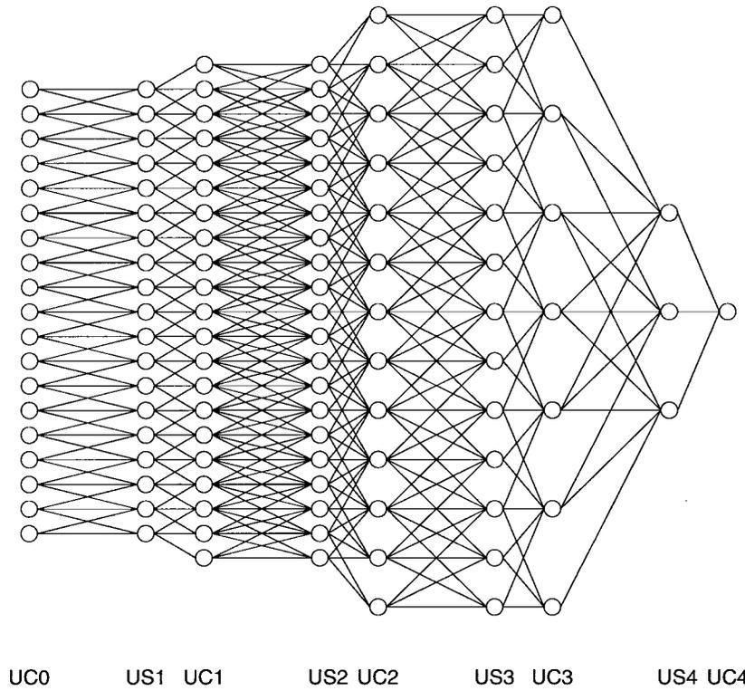
Fig. 5. This two dimensional “slice” through the neocognitron shows the interconnections between one S and C-plane from each layer of the network. It shows, for instance, how each of the cells in a  $13 \times 13$  layer 2 C-plane receives input from different  $7 \times 7$  cell regions in the preceding layer 2 S-plane. This figure is based on the network described in [3].
