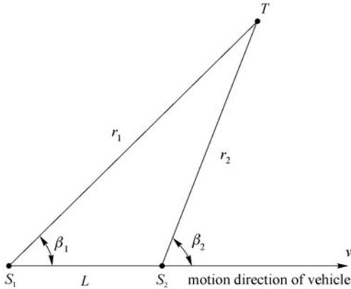
Fig. 1 Geometric schematic for airborne DF with single baseline
