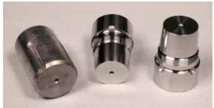
Figure #7; A2 tool steel test piece through hardened to RC 62. This test demonstrates hard turning of an interrupted cut, threading and contour machining.
