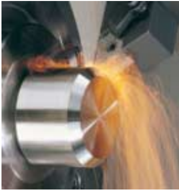
Figure # 1; Hard Turning on a Hardinge Quest lathe
