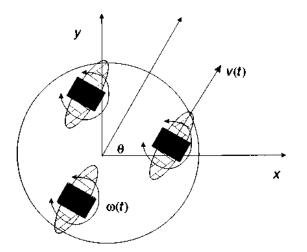
$$\begin{aligned} \mathbf{x}(t) &= \int_{0}^{t} \mathbf{v}(\sigma) \cos(\theta(\sigma)) d\sigma \\ \mathbf{y}(t) &= \int_{0}^{t} \mathbf{v}(\sigma) \sin(\theta(\sigma)) d\sigma \\ \theta(t) &= \int_{0}^{t} \mathbf{w}(\sigma) d\sigma \end{aligned}$$
