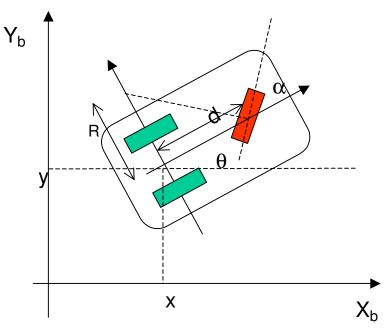
If the steering wheel is set to an angle  $\alpha(t)$  from the straight-line direction, the tricycle will rotate with angular velocity w(t) about a point lying a distance R along the line perpendicular to and passing through the rear wheels.
