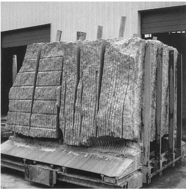
Fig. 2. Frame sawn granite slabs.
