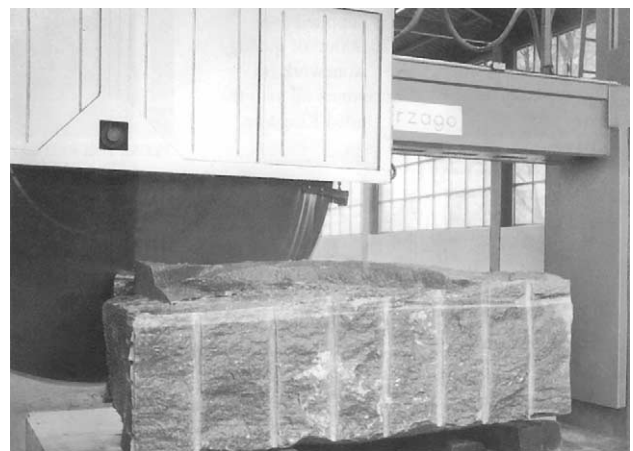
Fig. 5. Circular saw cutting granite.
