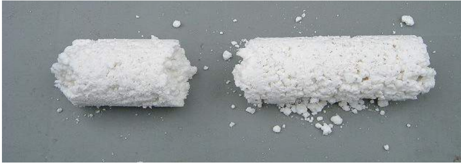
Figure 2 Granular emulsion explosives loaded to pipe (Loading density: 0.75 g/cm 3 )
