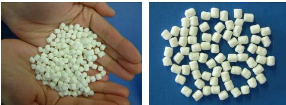
Figure 1 Granular emulsion explosives (Diameter: 4mm, Length: 4mm)
