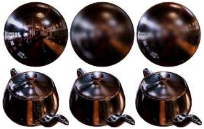
Figure 7: Variable glossiness reflections simulated with superposition of filtered environment maps. Left: sharp reflection. Middle: uniformly blurred reflection (Gaussian lobe). Right: blend between blurry normal reflections and sharp glancing angle reflection.
