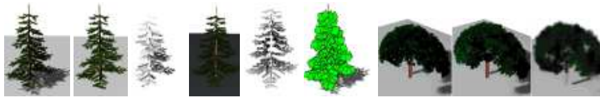
Fig. 7. Left to right: a pine tree with shadows, without shadows, amount of shadow. The pine with only ambient, the ambient visibility coefficient, the billboards used at the lowest level of detail. A prunus tree drawn at 3 levels of detail.
