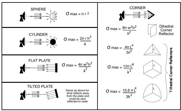
Figure 3. Backscatter From Shapes
