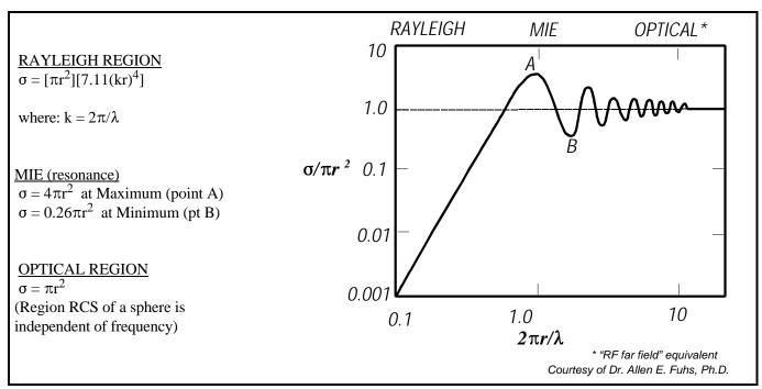
Figure 7. Radar Cross Section of a Sphere
