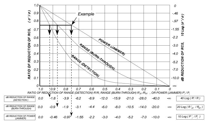
Figure 6. Reduction of RCS Affects Radar Detection, Burn-through, and Jammer Power
