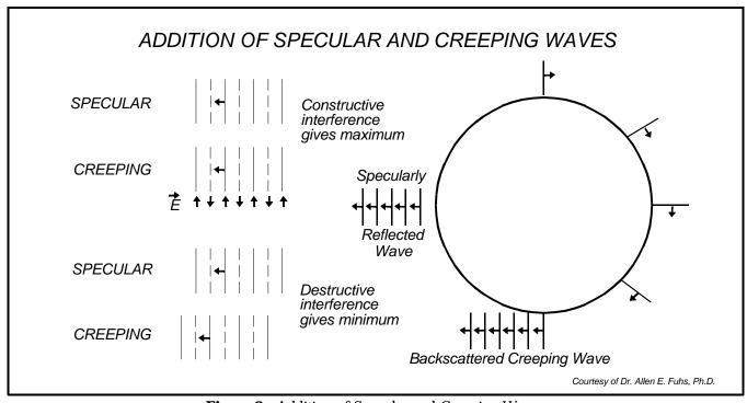
Figure 8. Addition of Specular and Creeping Waves
