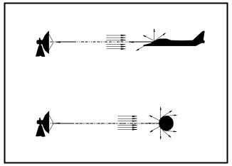
Figure 1. Concept of Radar Cross Section
