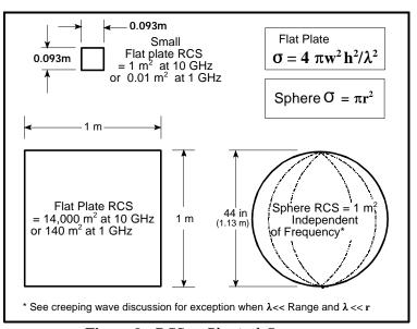
**Figure 2**. RCS vs Physical Geometry
