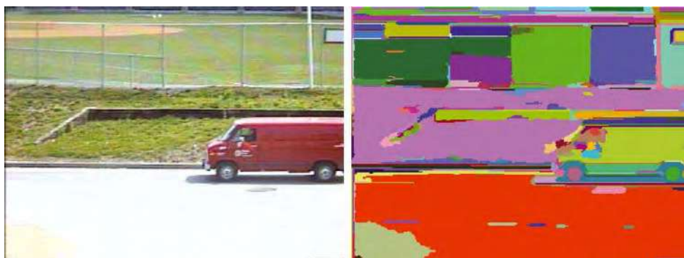
Figure 2. A street scene ( 320 \times 240 color image), and the segmentation results produced by our algorithm ( \sigma = 0.8, k = 300 ).
