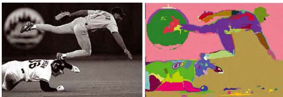
Figure 3. A baseball scene ( 432 \times 294 grey image), and the segmentation results produced by our algorithm ( \sigma = 0.8, k = 300 ).
