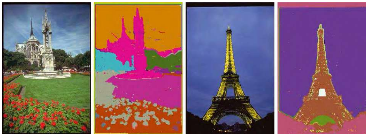
Figure 8. Segmentation using the nearest neighbor graph can capture spatially non-local regions ( \sigma = 0.8, k = 300 ).
