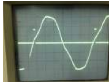
Figure 13. Experimental results of transformer output at A1 and monostable multivibrator U5 output at pin 3 [2v/div, 1ms/div].
