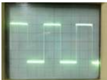
Figure 10. Experimental result of comparator U2 output at A3 [2v/div, 1ms/div].
