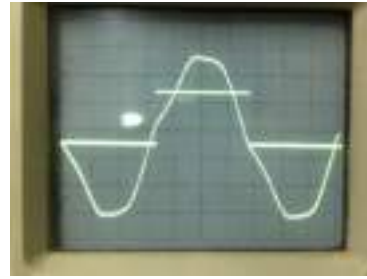
Figure 11. Experimental results of comparator U2 output at A3 and transformer output signal at A1 [2v/div, 1ms/div].
