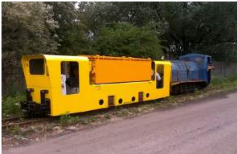
Fig. 8. Modernized Leabro BM-12 locomotive with transportation load in a form of diesel locomotive [7].
