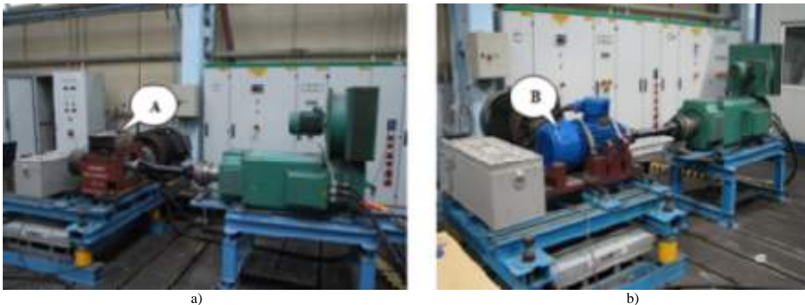
Fig. 3. Tests station [4]. A – brushless permanent magnet synchronous motor SMwsd 200 S-4, B – inductive motor dSkg 180L4-EP-f.
