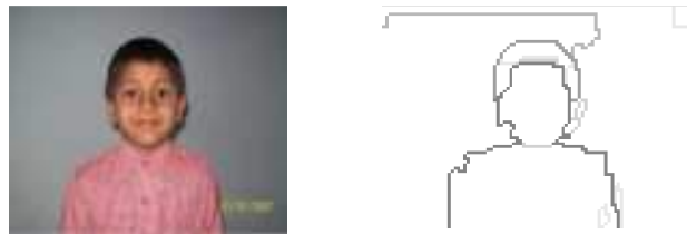
Original Image Region Based Segmentation Figure 1. Region based Segmentation
