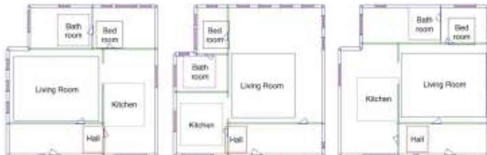
Figure 4: By placing some feature areas we can lay out the positions of rooms inside a building.
