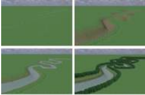
Figure 11. Creating a meander using natural systems: designing the shape in the game world then applying the height/soil, water and vegetation features [40].
