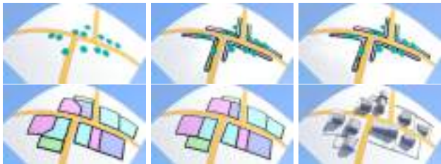
Fig. 7 Land parcels generation algorithm. From left to right: village skeleton, road conquest, corner conquest, region conquest, parcel simplification, building generation.
