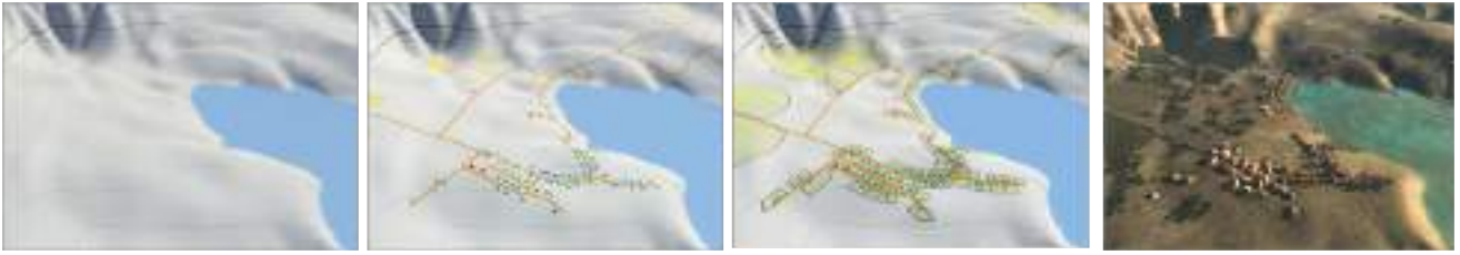
Fig. 2 Overview of our method: given an input terrain, we first generate the skeleton of the village (roads and settlement seeds), then we add parcels to the village layout, and finally generate 3D geometry for houses.
