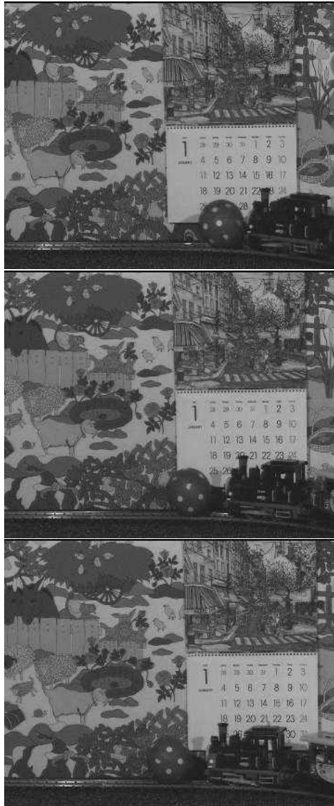
Figure B.10: Mobile - ( 720 \times 576 , 40 frames, 8bpp) This sequence contains motion of several independent objects and a slow camera pan.
